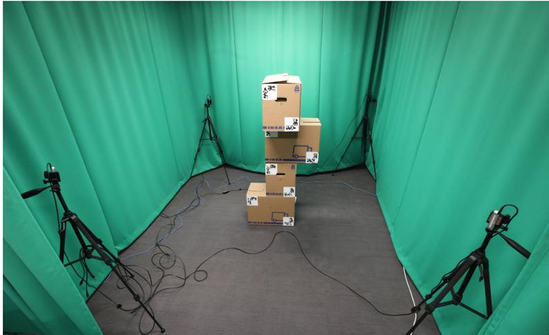
**Figure 1.3: Consumer-grade capture setup** This setup consists of four Intel RealSense D415 depth cameras mounted on tripods. The room is fitted with a green screen, to allow the background to be easily removed. In this picture, the cameras are capturing a stack of marked boxes, to facilitate the alignment process.
