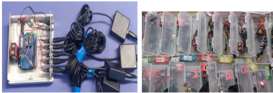
Figure 26 : Data gathering system. Our own built hardware to gather GSR data in the two scenarios (the 2 nd version hardware)
